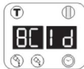
Then the display will show 8C-1D indicating that after every 24 seconds (shorten from 1D=24hours into 24 seconds) would automatically dose 8cc(ml) dosage. If you have collected 8cc(ml), this machine is functioning normally.
