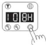
To begin quick test, press and hold "time setting" button
