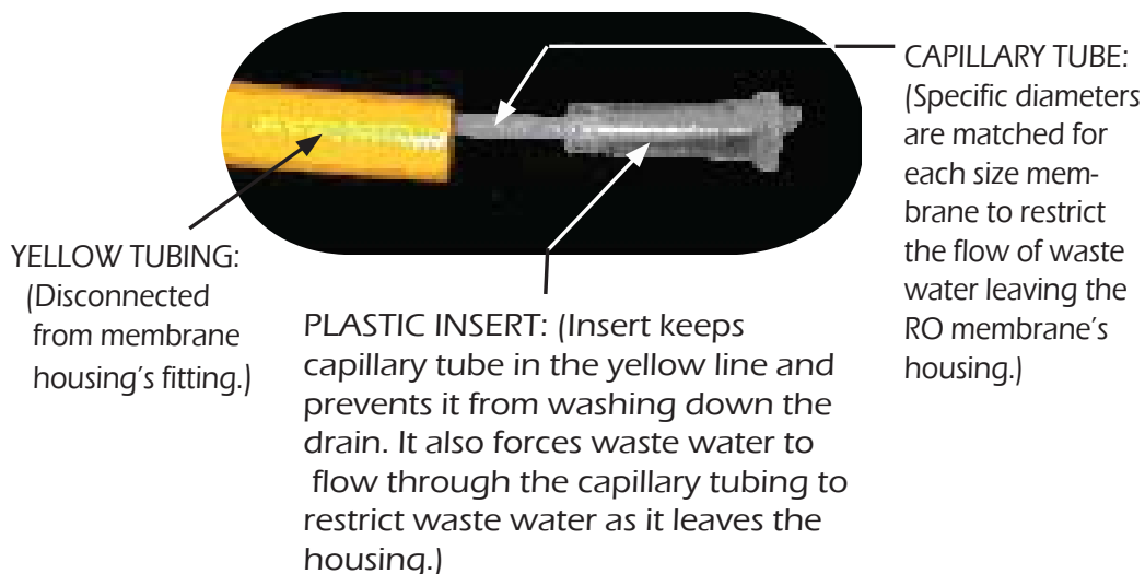
Fig. E: Flow Restrictor Assembly
